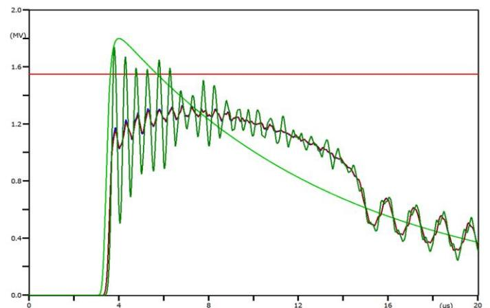
**Figure 7 Transient Voltages in the Substation with 30m Separation Distance**
