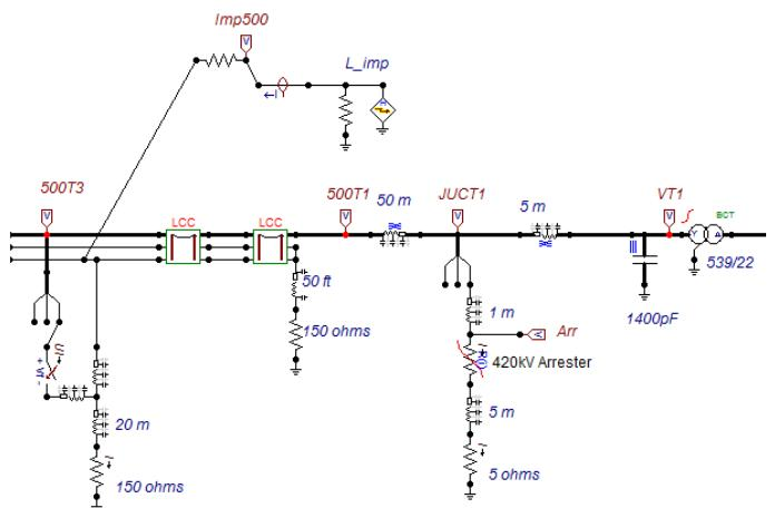
Figure 4 Circuit Modeled in ATP
