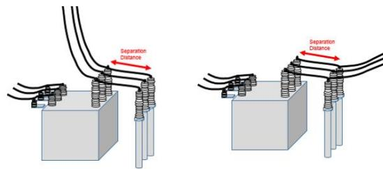
Figure B1 Arrester/Transformer Configurations with arrester before and after transformer
