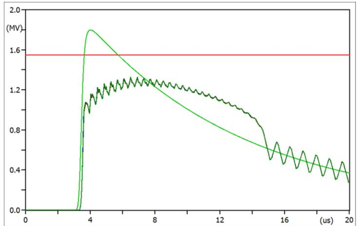
Figure 5 Transient Voltages in the Substation with 5 meters Separation Distance
