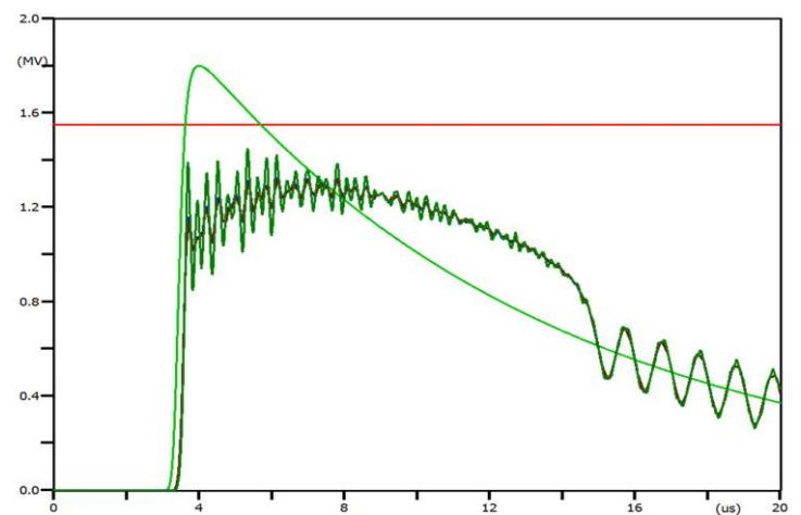
**Figure 6 Transient Voltages in the Substation with 15m Separation Distance**
