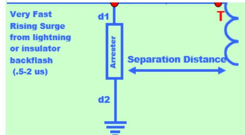
Figure A1 Circuit modeled in Calculator
